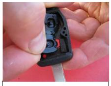
To fit new pad in you need to slide edge of round button under the coding chip first.
