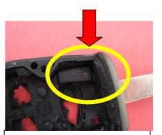
Important: please be careful not to damage Coding Chip located in the key part of the plastic cover at the bottom right corner
