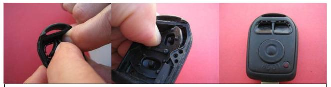
Once bottom button is fitted you will move to fit top buttons. You will be positioning one button at the time.
