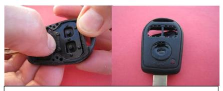
You have to push it in from inside the button using your thumb nail and manipulate it into position till whole button comes thru an opening.
