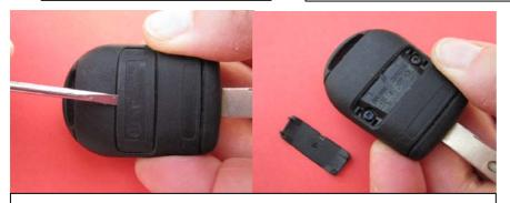
with flat screwdriver lift plastic cover positioned on the back of remote. You will uncover two screws which hold top and bottom part together
